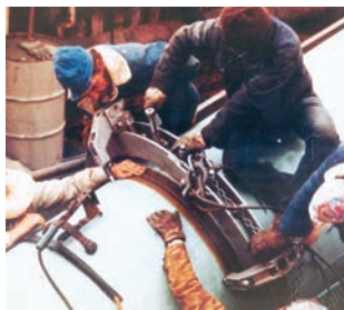
Mathey Dearman's Mega Rim Clamps are explicitly designed for the reforming of X65 or X70 pipe.
